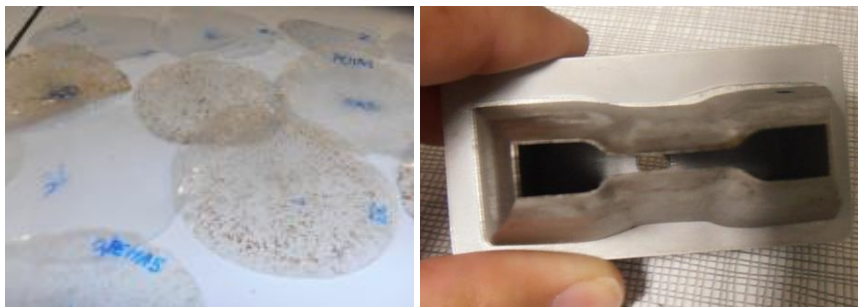
Figure 1. Films obtained from the rotomoulded parts (left); die used to obtain the test bars (right)
