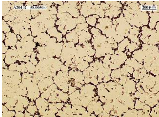
Fig.3: AlCu5MgTi (as cast). Grain size 125-200 μm
