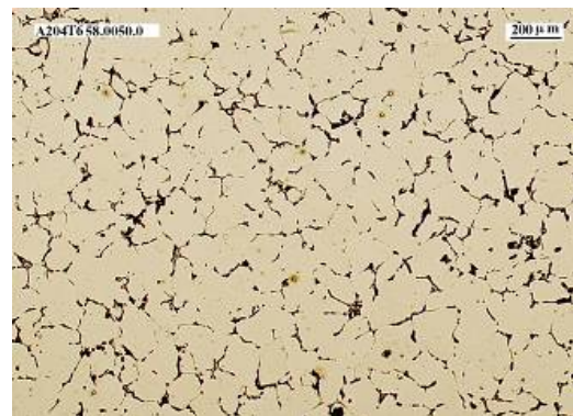
Figure 2: AlCu5MgTi (T6). Grain size 315-500 µm
