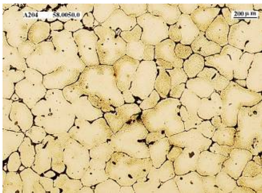
Fig.1: AlCu5MgTi (as cast). Grain size 200-315 µm
