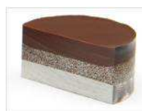
Figure 5. Image of PI/PI+Al/Al FGM cross section obtained by SPS.
