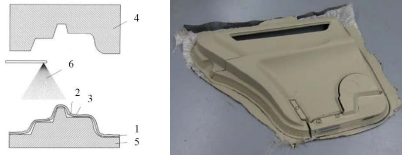
Figure 1. Illustration of the sandwich panel production process (left) interior side of a car door made from the presented glass fibre reinforced PU-foam sandwich panel with a PU imitation leather surface finishing (right).
