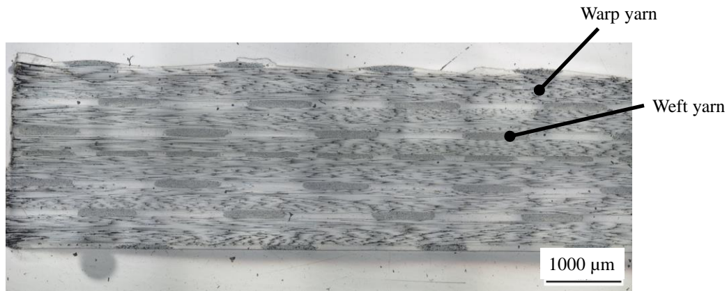
Figure 8. Optical microscopy image of the composite cross-section.
