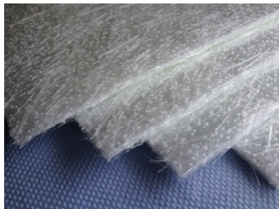
Figure 2. The plies of PP/GF19 vol. % (40 wt. %) hybrid mat
