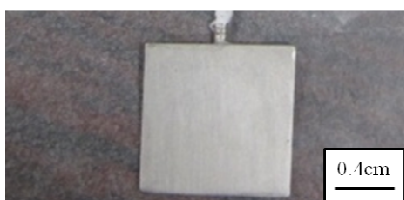
Figure 1. The deposited configuration of the electrospun membrane on the Pt electrode.
