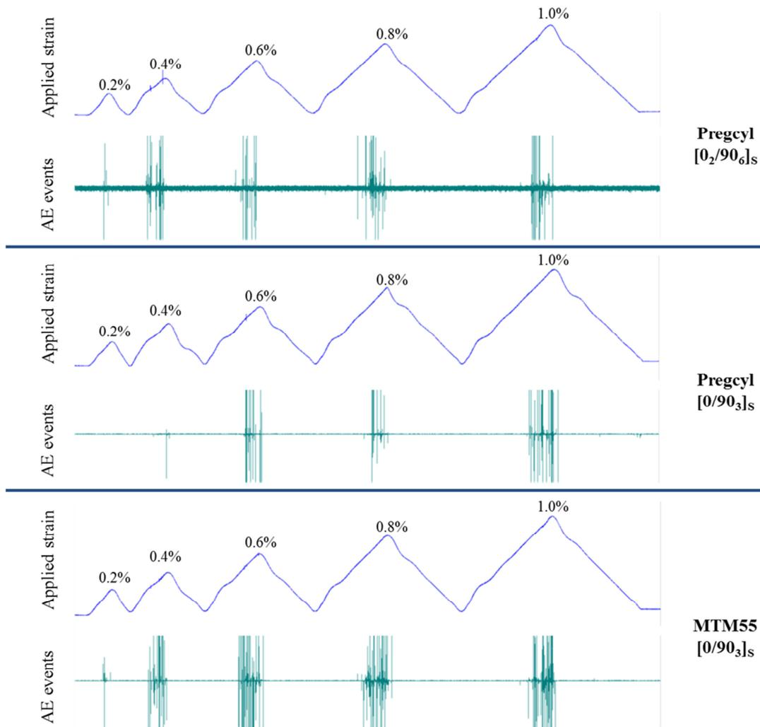
**Figure 5.** Applied strain as a function of time and corresponding AE response.
