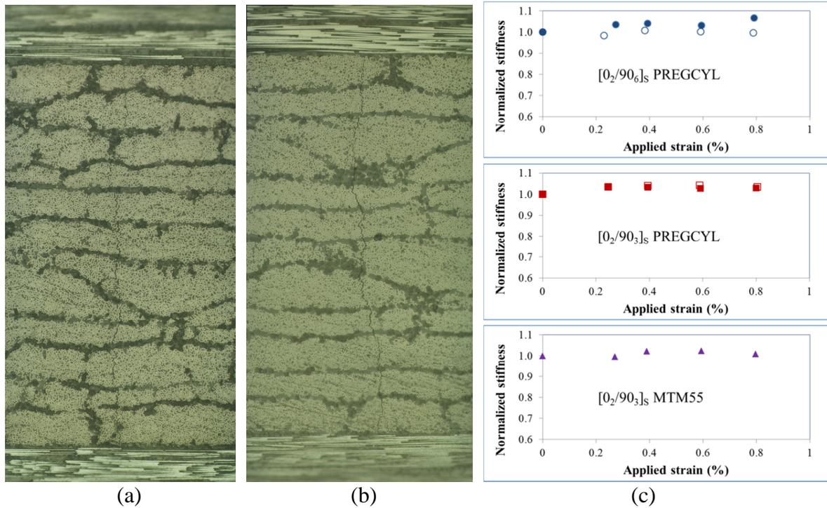
**Figure 6.** The micrograph showing crack in cross-ply laminate at 0.7% (a) and 0.9% (b) applied strain. The normalized stiffness as a function of applied strain for cross-ply laminates (c).
