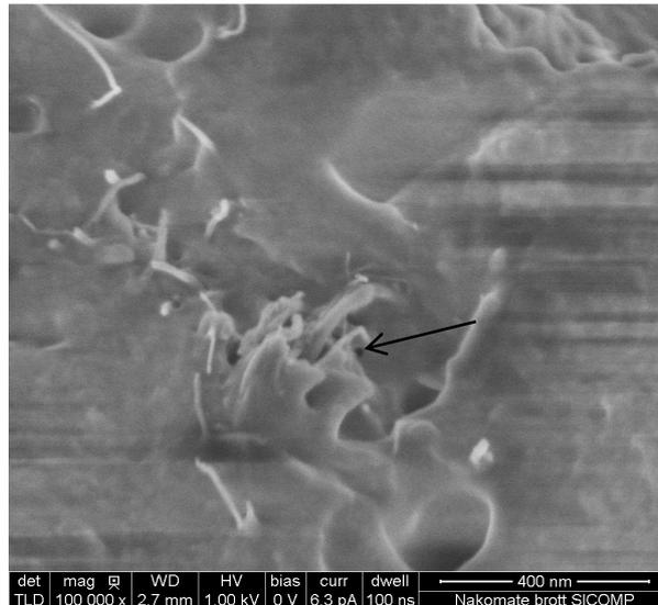
Figure 4. SEM-image of several CNT involved in fracture creating a brush-like appearance.
