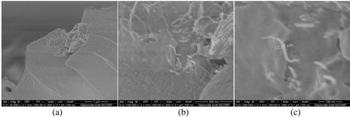
**Figure 2.** SEM micrographs with different magnifications from the same area of the fracture surface: (a) Shows a patch of CNT but also reveals that large areas lack CNT (b) Increased magnification of the patch shows that the dispersion is good (c) Dimension of an individual CNT.
