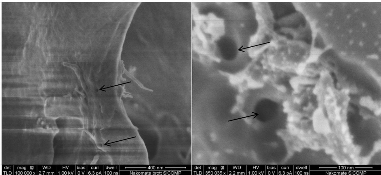
**Figure 3.** SEM-images of fracture surfaces of PREGCYL composites, arrows indicates traces from CNT-pullouts during fracture.
