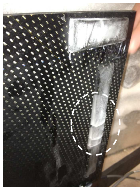
Figure 7. Cracked and semi-detached longitudinal ice-block.
