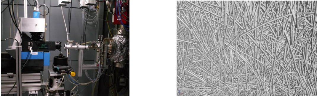
Figure 2. left – experimental setup of high resolution X-ray computer tomography at BESSY (synchrotron), right – high resolution (voxel size 0,4µm 3 ) CT-image of short fibers in tensile specimen
