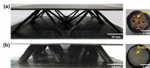
Figure 10. (a) Wood-core truss (b) silicone rubber-core truss and their corresponding carbon fiber composite pyramidal lattice structures.
