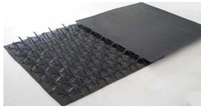
Figure 6. Photograph of a fabricated pyramidal lattice truss core sandwich structure
