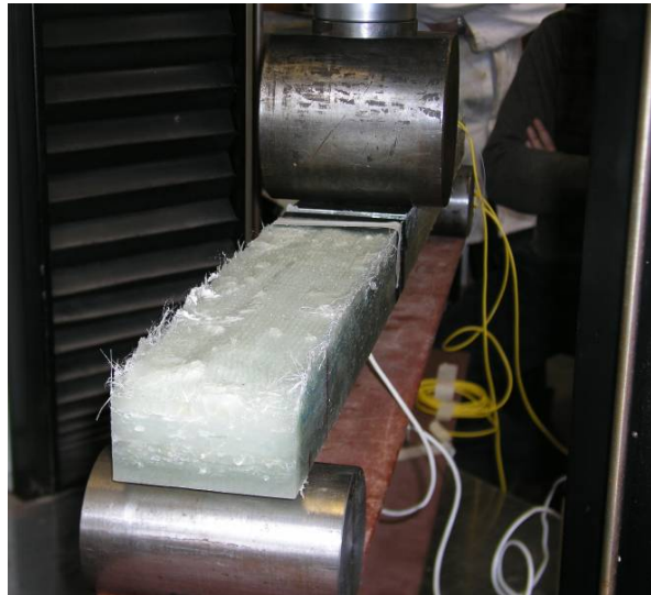
Figure 1. Three point bend test of thick beam
