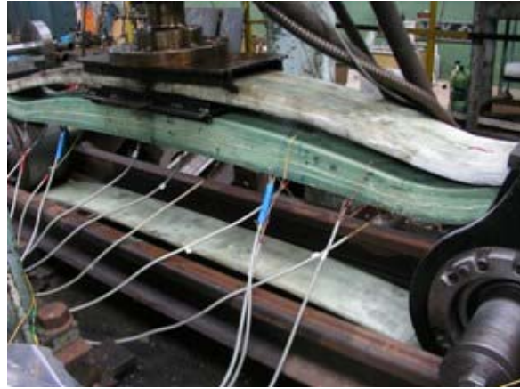
Figure 8. Side assembly bogie side undergoing testing
