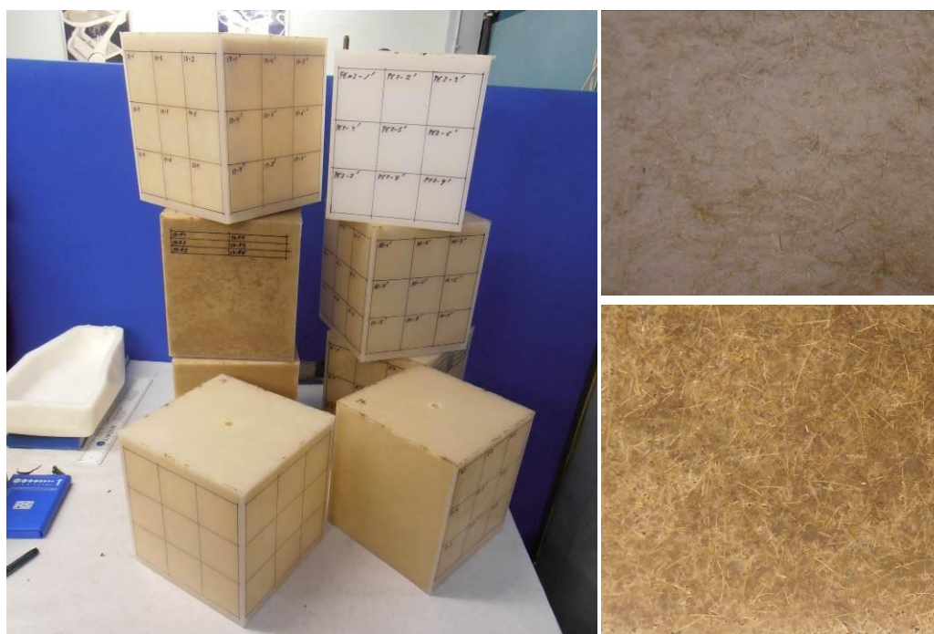
Figure 2. Some of test samples produced (left). PE 5 % BF before molding (upper right) and detail in one of the cubes produced (down left)
