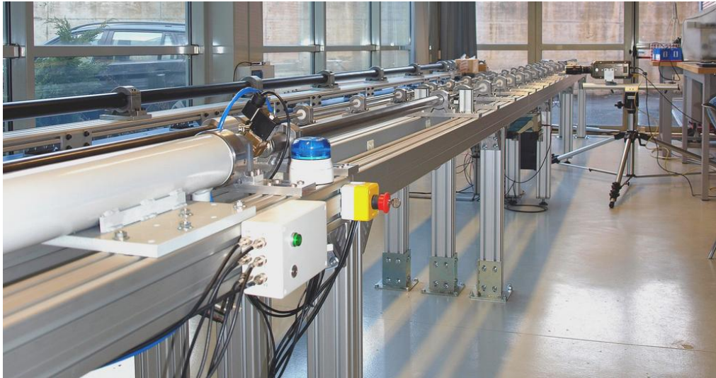
Figure 3. SHPB setup used for high dynamic tests.
