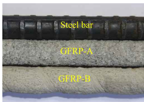
Figure 1. Surface deformations and type of bars.
