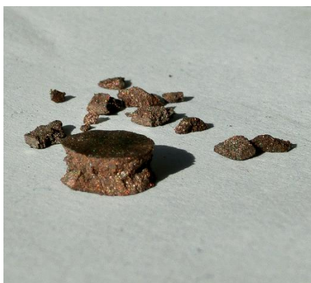
Figure 7. Picture of the cylindrical compression specimens used for quasi-static and high strain-rate tests (left); results in terms of maximum strength vs. strain-rate (right).
