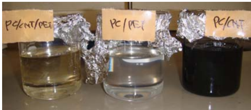
Figure 3. Photographs of the immerse experiments in chloroform; (left) PC/PET/CNT (44/44/11), (middle) PC/PET (50/50), and (right) PC/CNT (80/20).
