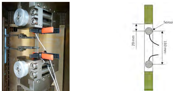
Figure 2. Static testing setup. Two AE sensors are clamped to the sample on defined positions. Strain is measured by an extensometer.
