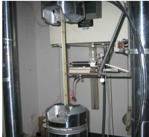
Figure 2. Testing apparatus for the buckling experiments of Glass/Epoxy beam specimen.
