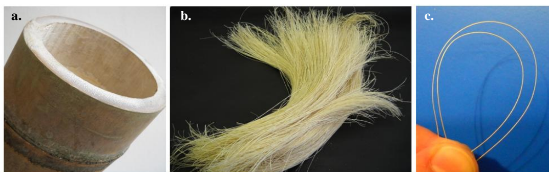
Figure 1. a) Bamboo Guadua angustifolia culm, b) group of technical bamboo fibres after extraction with an average diameter around 150 \mu\text{m} and a length of 35 cm and c) single fibres.
