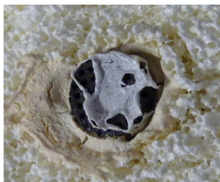
Figure 7: Pictures of a C/C coated with 10 layers coating after a cycle of 370 s, maximum temperature 1900°C.
