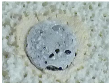
Figure 6: Pictures of a C/C coated with 10 layers coating after a cycle of 205 s, maximum temperature 2050°C.
