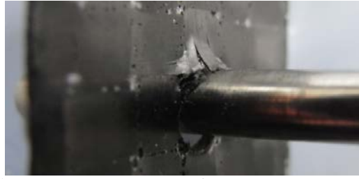
Figure 14. Fracture aspect of DH(PW) at D=4.0 mm
