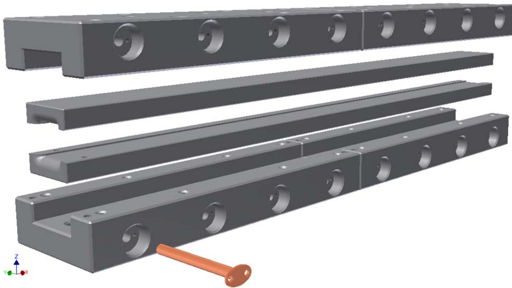
Figure 3: CAD design of the pultrusion die with die holder and heating elements.
