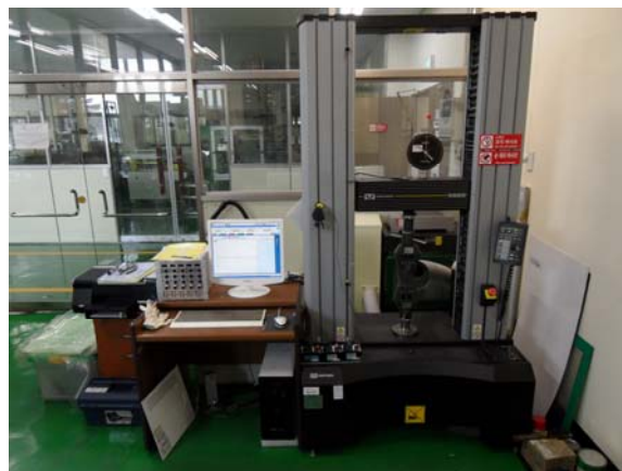
Figure 2. The universal tensile test machine for tensile tests.
