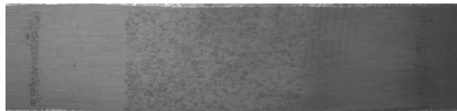
Figure 4. Yarn image as seen by the optical camera. Speckles on the surface are the binder particles. Full 5 mm yarn width is shown.
