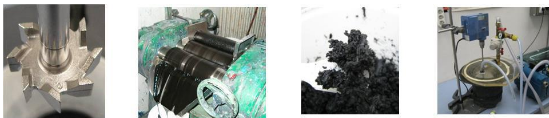
Figure 6: The steps of the masterbatch (MB) mixing technology: premixing by overhead stirrer, three roll milling, masterbatch, thinning under vacuum
