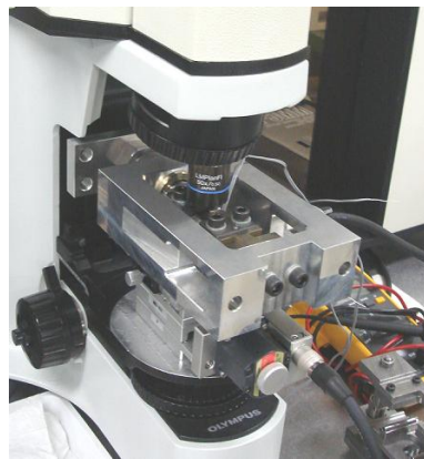
Figure 5. Micro-Raman spectroscope with a custom-made loading rig.
