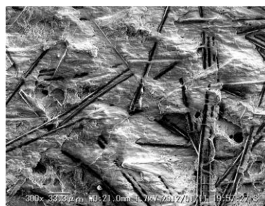
Figure 10. CMT/PP3 failure surface of single-lap
