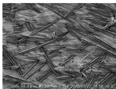
Figure 11. CMT/PP3 failure surface of scarf joint
