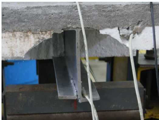
Figure 6. Failure in web profile for composite beams
