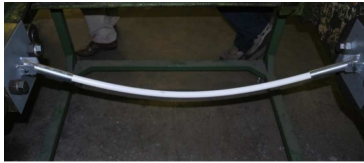
Figure 3. GFRP profile before failure under compressive and bending stress.
