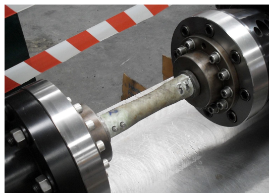
Figure 7. Torsion test of hybrid tubes
