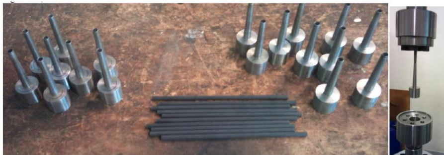
Figure 3. Carbon/epoxy rods, attaching parts, and testing systems
