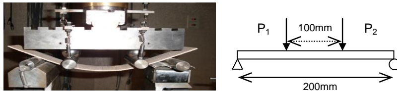
Figure 5: experimental setup four-point bending test
