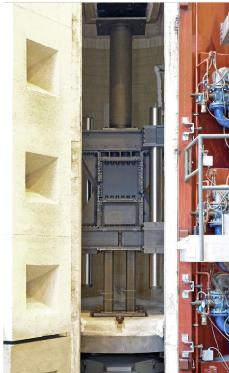
Figure 1: Test setup (compression device and furnace compression testing machine) with a carbon-FRP sandwich panel (500 x 500 x 20 mm)
