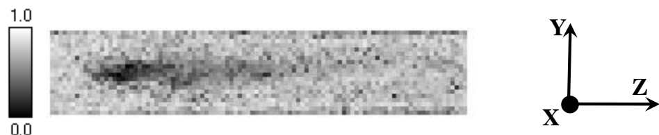
Figure 4 - Map of the value of the second order orientation tensor ( \langle \cos^2 \theta_x \rangle ) across sample A (YZ plane). The notch root is on the left.
