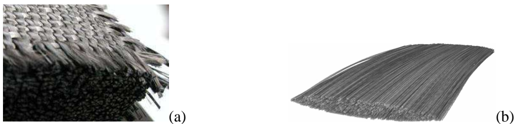
Figure 1. thick interlock (a) and the tomography of a single yarn (b)
