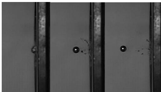
(a) Single fabric C Figure 10. Sequence of single-ply fabric deformation and failure for impact velocity 263 m/s
