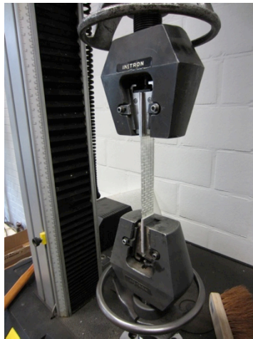
Figure 1. (left) Tensile test set-up for a UD glass-fibre material. (right) Stress-strain curve from a tested sample
