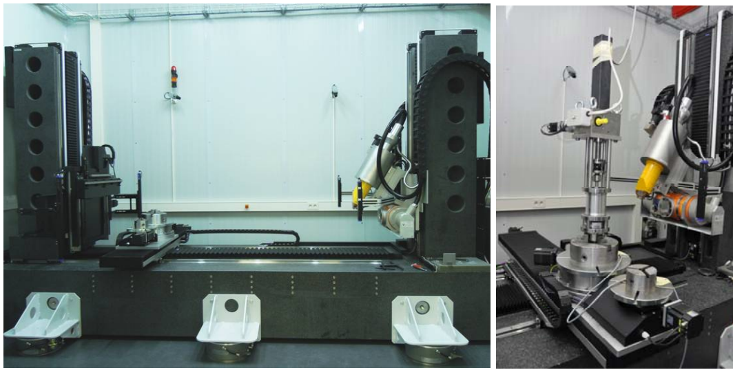
Figure 1. Computer tomograph V|tome|x-L 450 (left); In situ CT test device (right)
