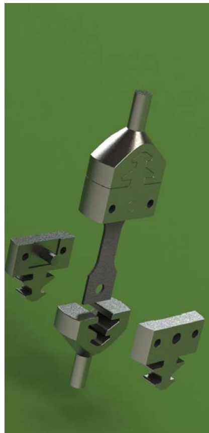
Figure 3. Clamping system for in-plane loading
