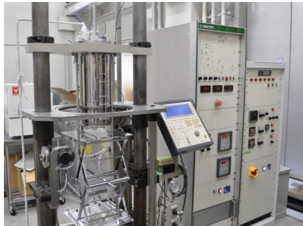
Figure 1. Materials testing system simulating a severe environment. System consists of a materials-testing machine, pressure vessel, environmental simulator and PC controller.
