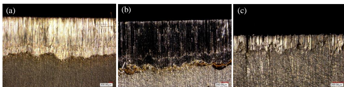
Figure 3. Observation of the cutting edge of (a) 0.8kW CO 2 laser-cut, (b) 0.3kW fiber laser-cut and (c) 2kW fiber laser-cut .
