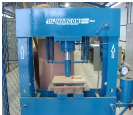
Figure 3. Composites manufactured using the compression molding technique.
