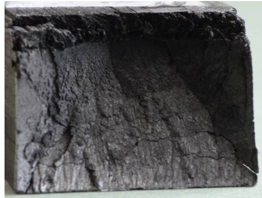
Figure 12. Failure area of the sample from high modulus fiber K63712
