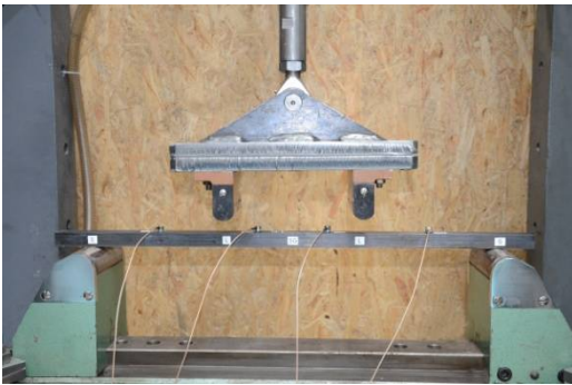
Figure 3. Four-point bending (4PB) test configuration.
