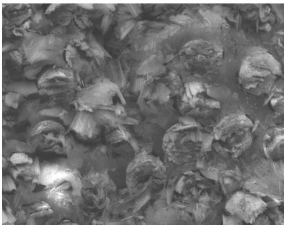
Figure 14. Failure area resulting from measuring of static strength
