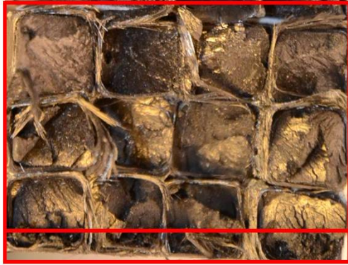
Figure 11. Failure area of the sample K63712/T700. Red rectangle pointing out compressive and tensile failure mode
