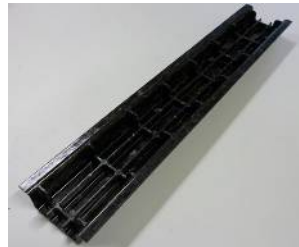
Figure 4. CF/PP hat-channel reinforced by 10 mm high ribs.
