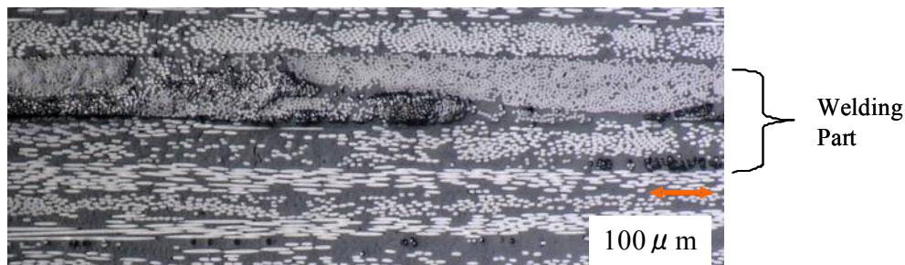
Figure 2. Welding zone observation of beam A-1 by optical microscope.
