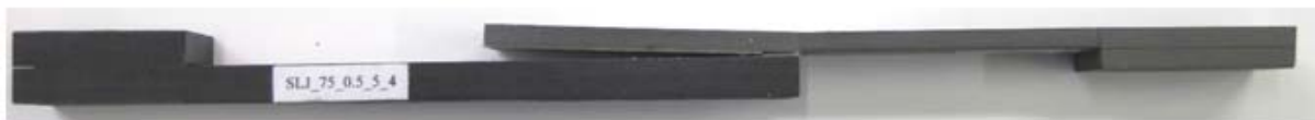
Figure 9. Typical failure mode of a specimen of the SLJ-3 or SLJ-4 case denoting permanent plastic deformation of the steel substrate
