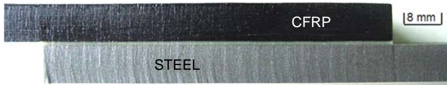
Figure 3. Side view of a typical SLJ with 75 mm overlap length.
