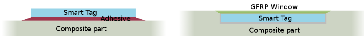
Figure 1. Possible configurations for the integration of Smart tags on the composite structure
