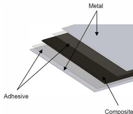
**Figure 2.** Laminate stacking configuration
