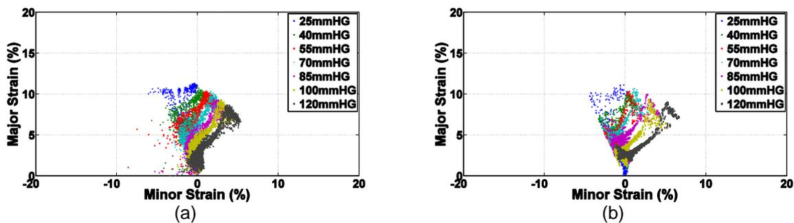
Figure 8. Forming limit diagrams for the experimental geometries (a) and the finite element simulation (b)
