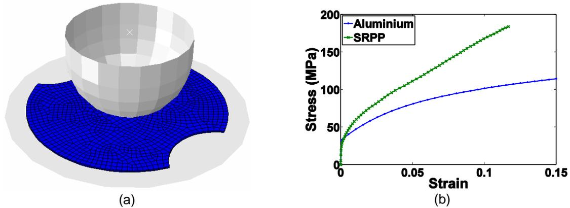
**Figure 4.** Finite element model (a) and the stress-strain relationship for the materials (b)
