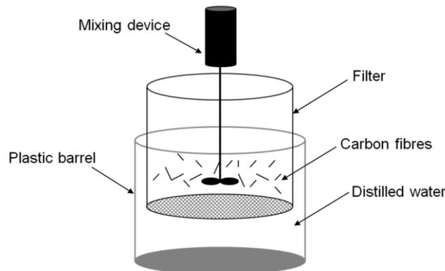
**Figure 2.** Dispersion of the recycled carbon fibres.
