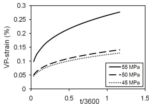
**Figure 7.** Predicted evolution of VP-strains with time in creep tests.
