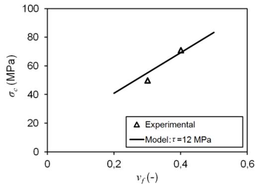
**Figure 6.** Experimental and modelling results of the strength of the rCF/rPP composite.
