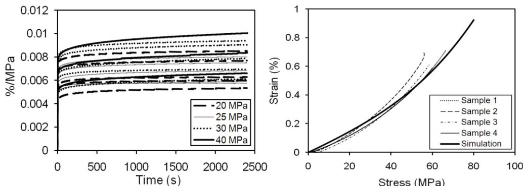
**Figure 8.** Viscoelastic results: **a)** creep compliance at different stress levels, **b)** experimental and predicted constant stress rate loading curves at a stress rate of 1.0 MPa/min.
