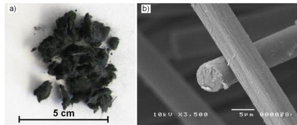
**Figure 1.** Recycled carbon fibres: **a)** cotton-like structure, view with the naked eye, **b)** individual fibres (x7.5k).
