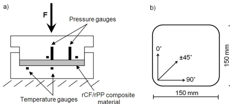
**Figure 3.** a) Matched die tool used to manufacture the recycled polypropylene films and the composite material, b) top view of manufactured plates showing the cutting directions of the samples.
