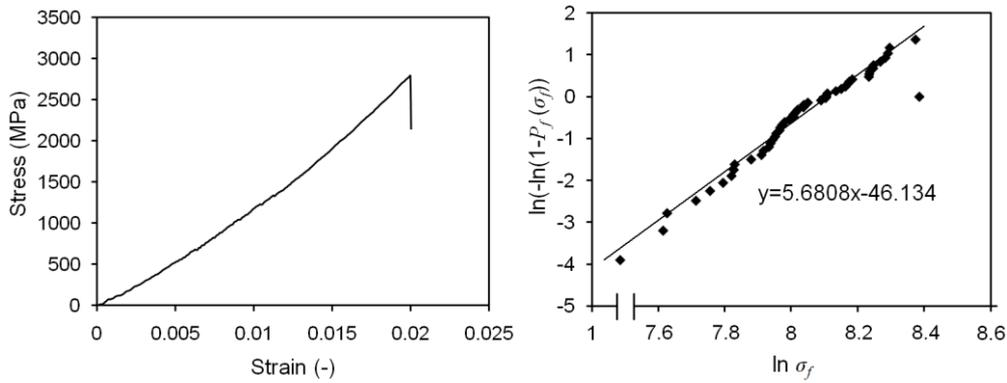
**Figure 4.** Single fibre properties: **a)** typical stress-strain curve of a single rCF, **b)** strength distribution of the rCF using a 10 mm gauge length .
