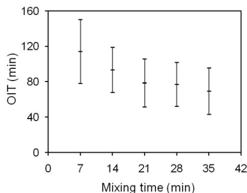
Figure 4. Oxidation induction time results for the PP scrap.
