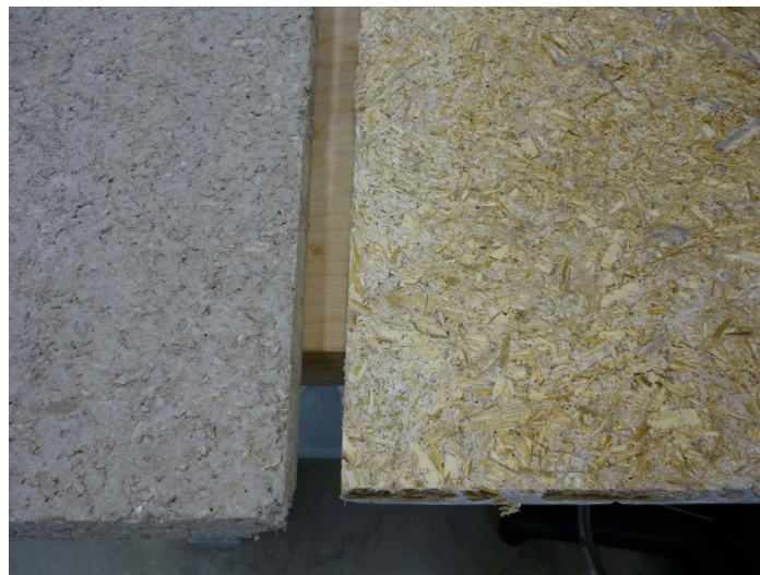
Figure 4. Hemp based panels for thermal conductivity tests: RT-1 (on the left) and MC-2 (on the right).
