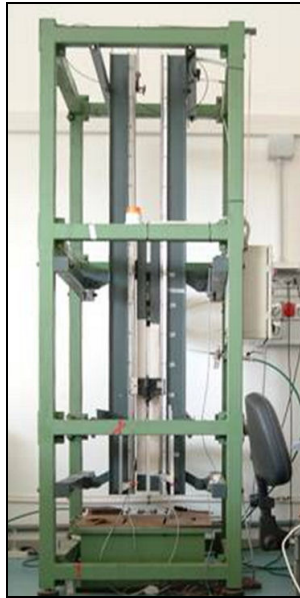
Figure 10. Tooling for the impact tests
