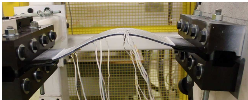
Figure 8. Deformed shape of repair evaluator just before final collapse.
